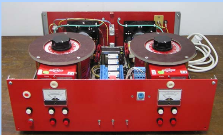
One of the 3 power and control modules for two magnetrons, in various stages of execution
